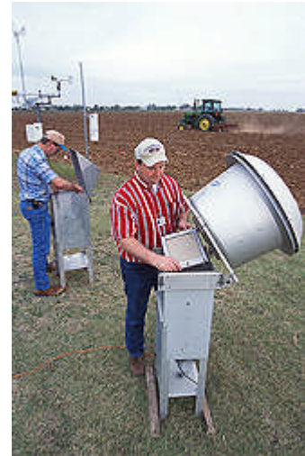
Agricultural engineers Greg Holt (left) and former ARS scientist Michael Buser, now with Oklahoma State University, Stillwater, change filters from particulate-matter samplers and collect meteorology data while sampling dust generated by a rolling cultivator (background).
