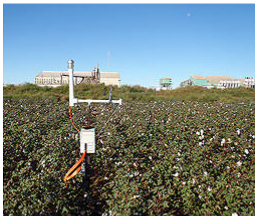
ARS scientists measure the levels of PM 2.5 and PM 10 in the air outside a cotton gin by surrounding the gin with 126 ambient air samplers, such as this one located in a cotton field near a cotton gin in west Texas.
